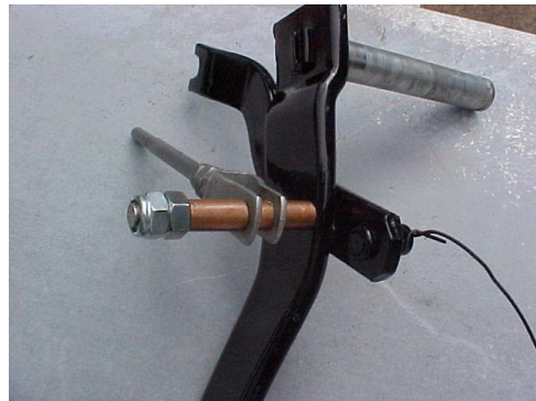
Push rod attached to the clutch pedal. The wire in the picture was for hanging the pedal to allow the new paint to dry.
