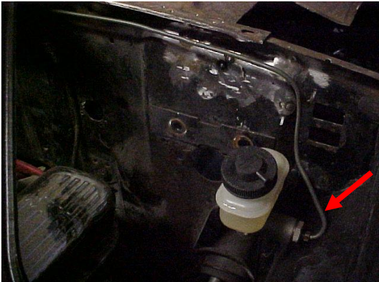
Looking down on clutch m/c. The hydraulic line is very close to the inner fender on the right. Also notice that the cowl is apart for repair leaving a nice access hole for the trial fitting.
