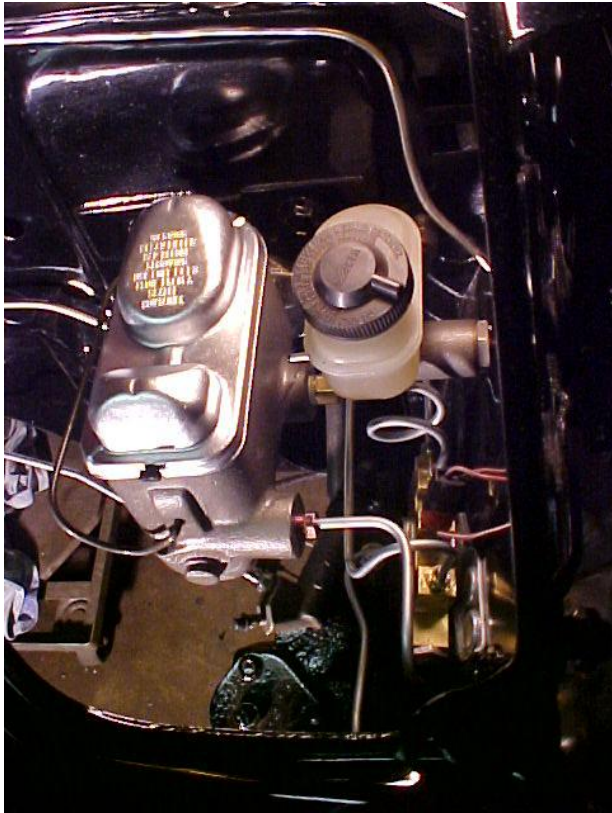
Looking down on clutch m/c. The hydraulic line is very close to the inner fender on the right. Also notice that the cowl is apart for repair leaving a nice access hole for the trial fitting.
