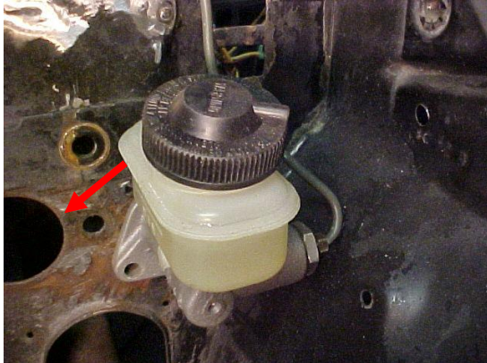
Close up of the clutch m/c; notice the hole for the brake m/c to the left.
