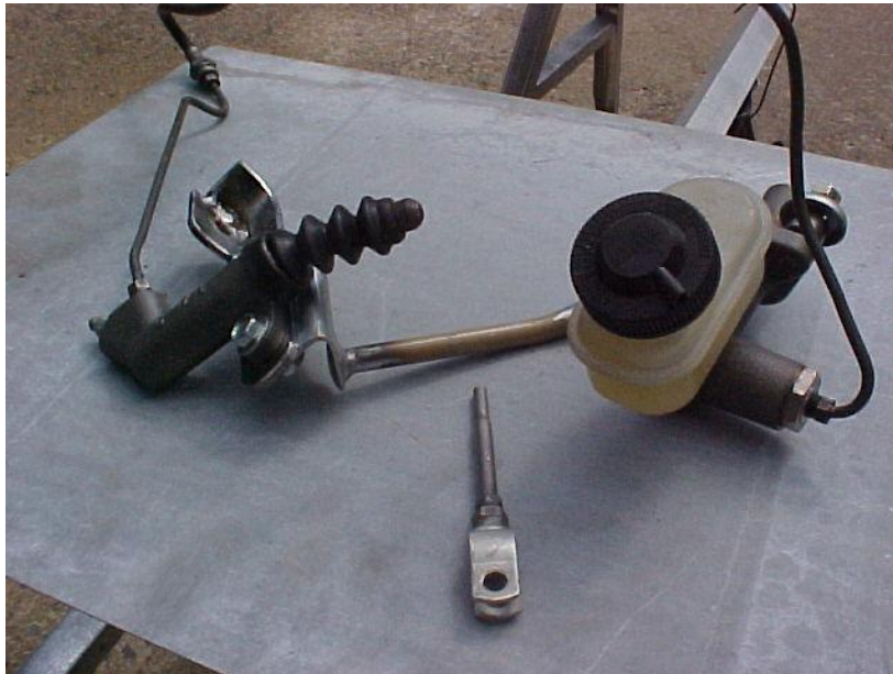
1991 Mazda 626 clutch master cylinder, slave cylinder, hydraulic hose and push rod. Attached to the slave cylinder is the fabricated bracket.
