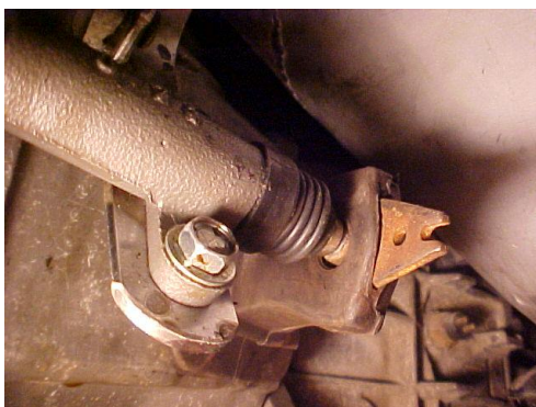
The slave cylinder pushes against the clutch fork.
