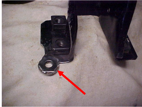
A washer was welded on the pedal support bracket to relieve stress on the firewall.
